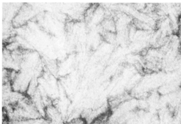
Figure 5. Texture of polymer I at 152 °C. Crossed polarizers; original magnification 200 \times (the photomicrograph has been reduced to 60% of the original size for publication purposes).
