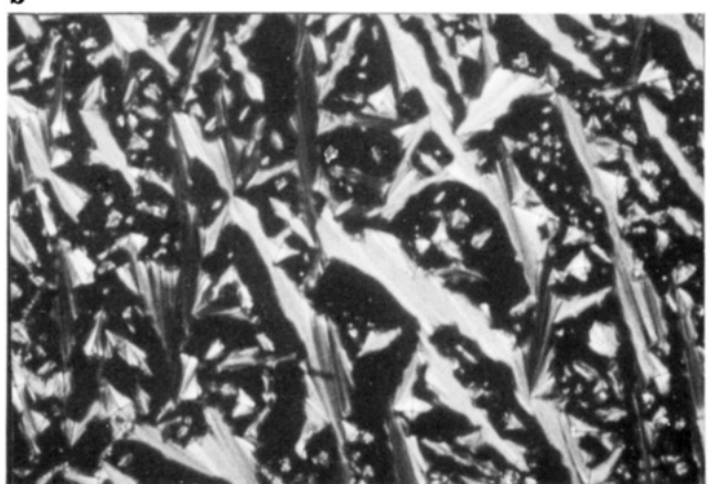
Figure 3. Separation of the smectic phase in the form of batonnets from the isotropic liquid of polymer I: (a) 167 °C; (b) 162.7 °C. Crossed polarizers; original magnification 200 \times (the photomicrographs have been reduced to 60% of the original size for publication purposes).
